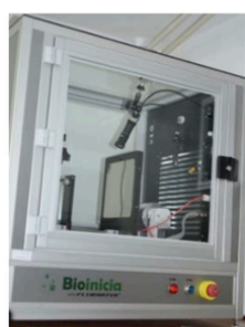
Sistemul de electrospinare Fluidnatek
